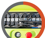
Lead acid battery
